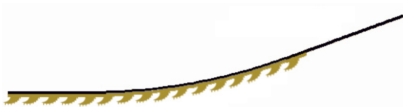
Figure 9. Concept drawing of "hairy" anisotropic rear foot.
